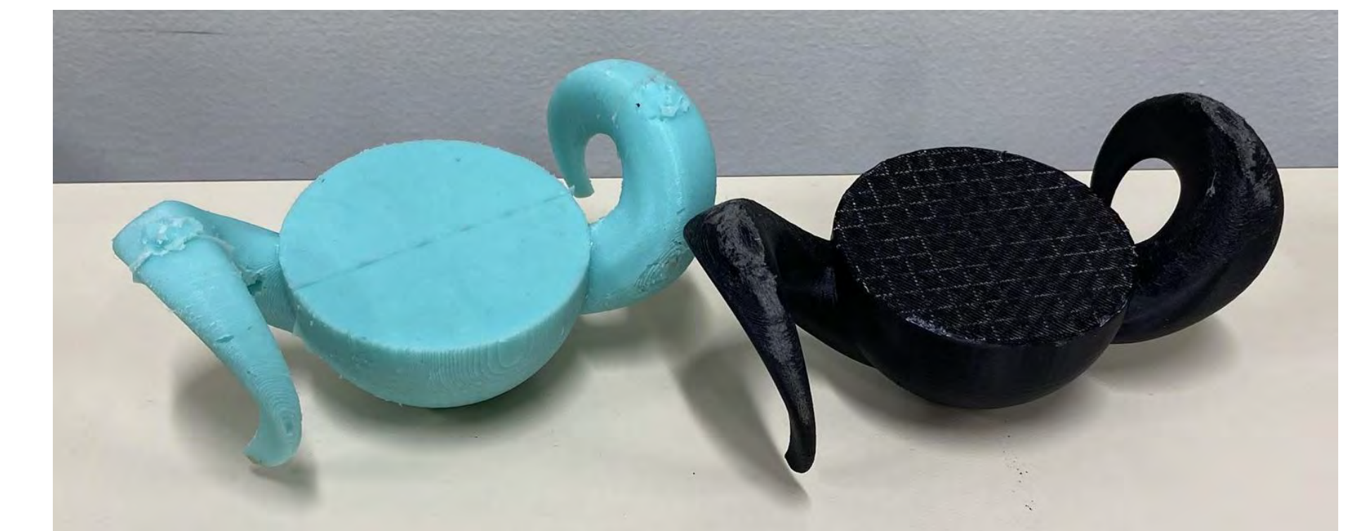
Figure 5. 3D printed 2 horn-impactor geometry and its corresponding silicone cast.
