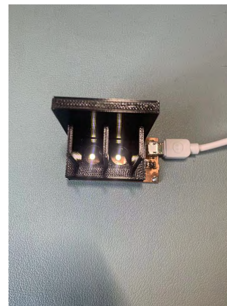
Figure 2. 3D-printed container for holding water samples
